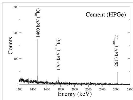
**FIGURE 1.** A gamma-ray spectrum of a Portland Cement sample analyzed.
